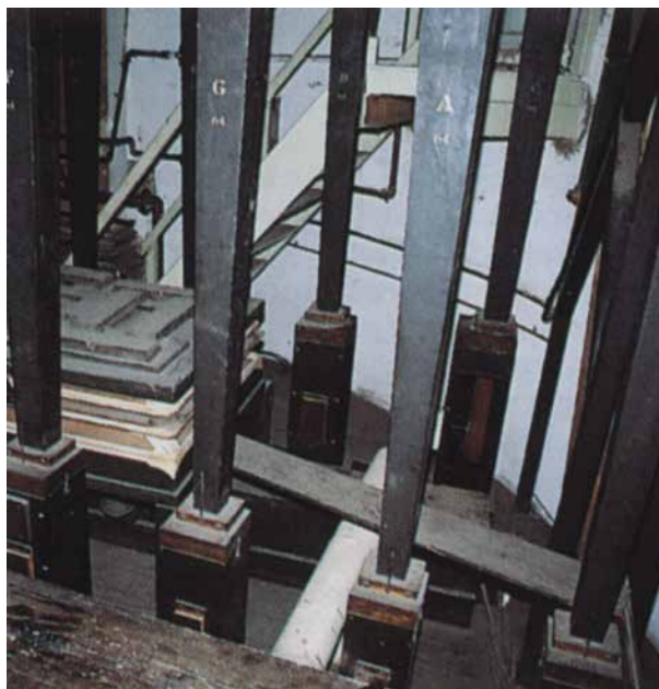
PIPES FROM THE BOTTOM OCTAVE OF THE PEDAL 64' STOP WITH THEIR OWN WIND RESERVOIR.
