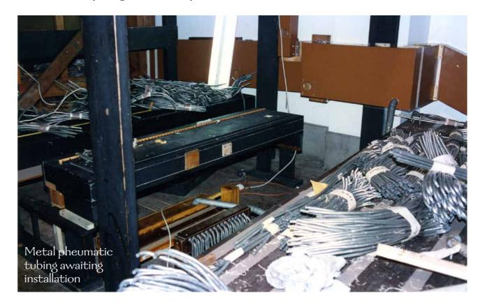
pneumatic motors and valves; also some of the metal pneumatic tubing had been crushed underfoot and numerous connections had come apart. The pipework was in reasonable condition, given its age, and was only superficially damaged, although very dirty, affecting the speech, regulation and tuning. The console had sustained considerable wear and a number of ivory keys, together with many pedal keys, were badly worn and the casework and facade pipes were grimy.
